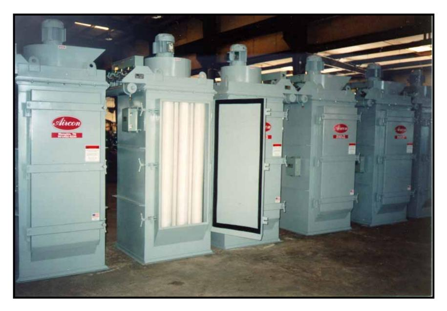
BIN VENTS - STANDARD ORIENTATION TOP-MOUNTED FAN, BOTTOM BAG REMOVAL w/ HINGED ACCESS DOOR
